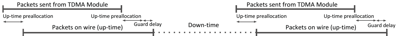
Figure 3: A TDMA schedule. Up-time preallocation and guard time correct for observed delays and variance in packet transmission from NIC hardware.
