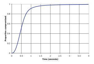
Figure 6: Proportion of one million and eighty hosts compromised by fast TCP worm as a function of time.
