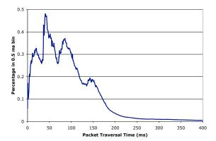
Figure 3: Histogram of globally averaged Internet latencies for February 2004 as determined by CAIDA's Skitter infrastructure. See the text for details.
